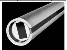
**Type AM Core** (to fit Airmaze Roll-A-Maze). Core is formed from fiberboard tube with 1-7/8" I.D. tube has recessed cups secured in each end with adepth of 5/8". Cup is stamped to form a 1-1/2" x 3/4" rectangular slot.
