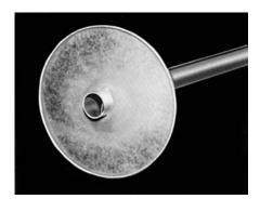
**Type B Core** (to fit BLC Industries Automatic Roll Machine). Core is constructed from 1-1/2" diameter: EMT conduit, with 11" diameter end plates recessed in approximately 1-3/8" from end of core.
