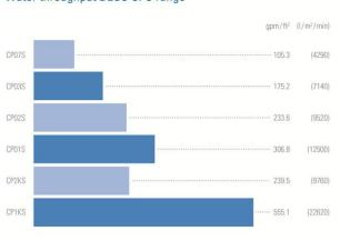
Conditions:  $\Delta$  p = 14.5 psi (100 kPa, 1 bar), Medium: Water at 68 °F (20 °C)
