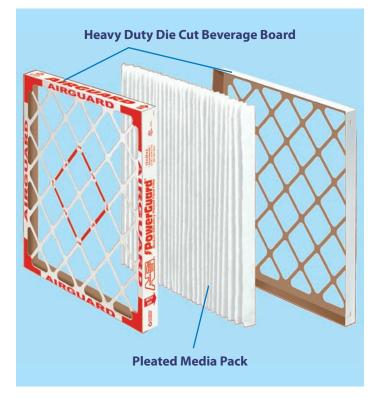
Two mating pieces of die cut beverage board form a double wall frame around the perimeter of the filter. PowerGuard filters will not rack or warp under normal operating conditions.
