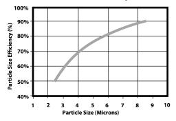
1. Efficiency - MERV 8 Performance (ASHRAE 52.2-2007). Data based on 24x24 and tested at 492 FPM
