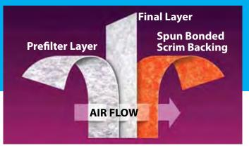
Vari-Pak Model S dual layer synthetic media has a built in prefilter layer consisting of coarser fibers followed by a high efficiency final filter layer made of microfine fibers.
